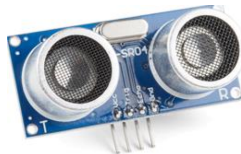
Figure 2: An Image of an HC-SR04 Module (Core Electronics, 2022)
