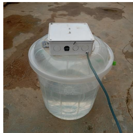
Figure 9: The picture of the fuel level monitoring and notification system casing.
